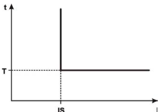
Figure 4 Principle of protection with an independent time delay.
