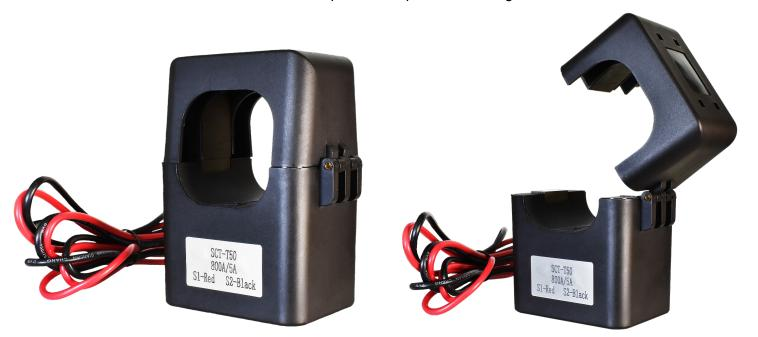
A bus or cable is passed through the opening of the magnetic circuit, which serves as the primary winding of the product. For ease of installation, the magnetic circuit is made detachable. The product is fastened to the
